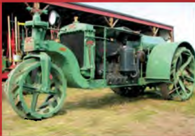
Samson tractors were noted for their unique wheels that gripped Midwestern soil without becoming mired in it. Courtesy of Bernie Smith.
