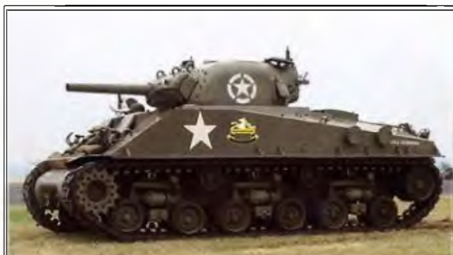
An early M4 Sherman Medium Tank. Note the similarity in the frontal armor shape with the T-34. The early Shermans had 75 millimeter guns that lacked the velocity and mass needed to penetrate the frontal armor of German tanks.
